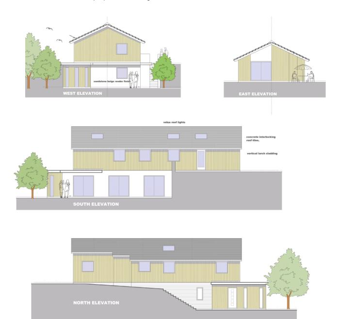
6.19 The dwelling will be constructed from cream render and vertical timber cladding on the elevations with concrete interlocking tiles on the roof and a sedum roof on the single storey
